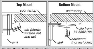
**For Top Mount:** Positive holddown clamping twist-tabs designed for up to 1" (25mm)-thick countertops. FOR COUNTERTOPS THICKER THAN 1", CONTACT FACTORY.
