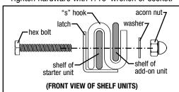
Repeating Steps 1-3, install additional Security S-Hooks as desired.
