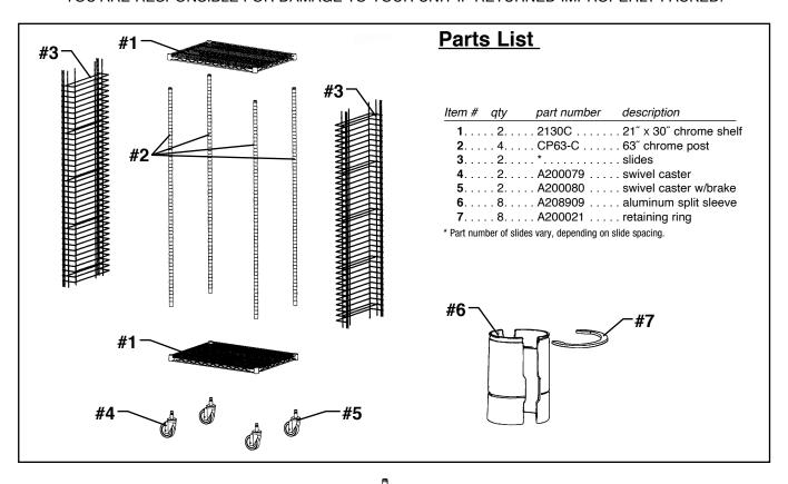
Step 1 - Attach caster to bottom of each post.
