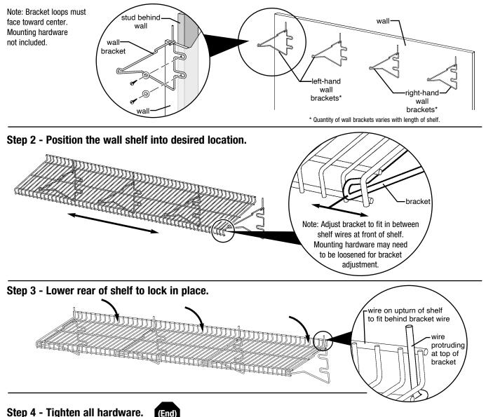
Note: Wall mounted units must be attached to a properly constructed and sound wall. For walls constructed of wood or steel studs, the mounting points must be directly on the stud or suitable in-wall-grounds of plywood or sheet metal. Eagle Group cannot be held responsible for the failure of the device or any other devices due to improper installation.
