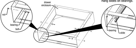
Step 5 - Attach drawer enclosure to hat channels underneath adjoining table.
