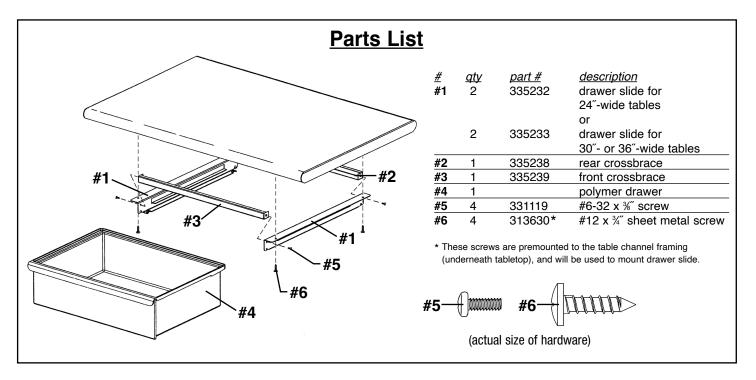
Step 1 - Attach crossbracing to drawer slides.
