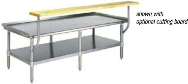
Eagle's Griddle/Equipment Stands feature patented uni-lok® system: Gussets are recessed into hat channels that run underneath stainless steel tabletop, reducing lateral movement. 1-1/4" high upturns run along the rear and both ends of the tabletop. Adjustable undershelf. 1-5/8" diameter legs with adjustable metal feet.
