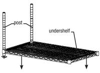
**Step 5: Secure undershelves.** Note: Do NOT hammer directly on wire
