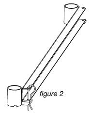
3) To prevent totes from sliding out, install the hook into the hole of top flange and push downward to secure. Slot will capture shank of hook when properly installed. See figure 2.
