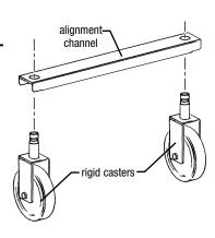
Step 3 - Drive in caster using a hammer or mallet.
