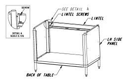
(5) Secure table top to legs by tightening set screw\* with allen (hex) wrench. Typical (4) places (lintel not shown for clarity).
