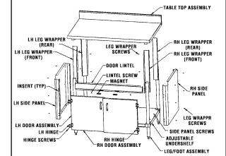
(2) Slide side panels over leg/foot assemblies and attach with screws.
