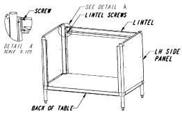
(5) Remove sheet metal screws from the front tabletop channel only.
