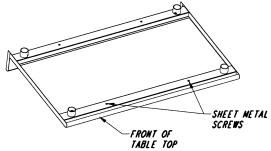
(6) Re-install the sheet metal screws thru the designated holes in the lintel. The holes should match with leg channel holes (diagram shows back side of lintel).
