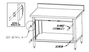
(8) Diagram shows all leg wrappers in place with screw placements. Six screws secure each leg wrapper (some screws not shown).
