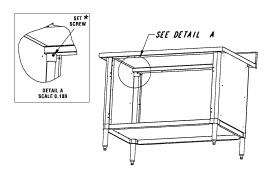
\* To meet NSF standards: Set screws must be filled with NSF-approved sealant. set screw
