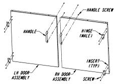
(12) Install right and left hand door assemblies by sliding (male) pinned hinges on doors to female hinges on side panels.
