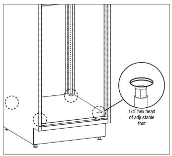
**Step 3:** At each leg, using a 1/4" socket, turn hex head bolt to adjust height of foot.
