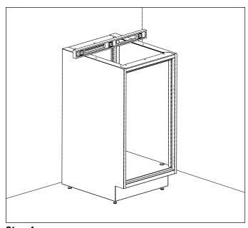
**Step 4:**Adjust feet until cabinet is level front-to-back and side-to-side. When adjustments are completed, return plastic caps.
