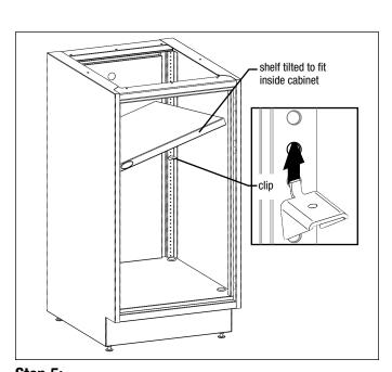
**Step 5:**To install shelf, tilt shelf to fit inside cabinet. Install shelf clips at desired height, and place shelf on top of clips.
