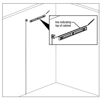
**Step 1:**Measure and mark desired height of overhead cabinet. Use a level to extend line.
