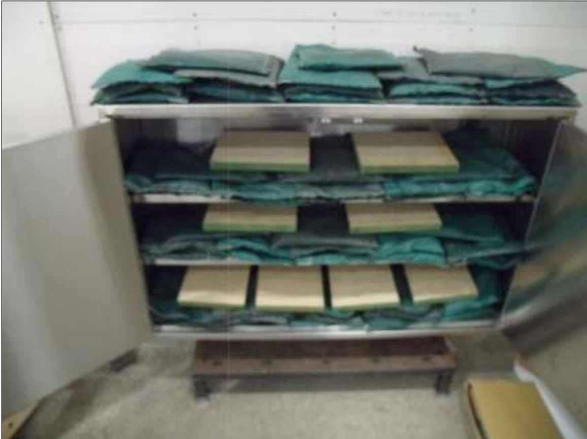
Wall Mounted Cabinet Load Test
