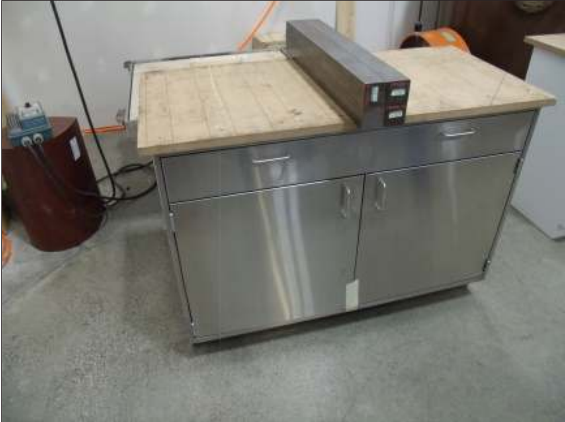
Cabinet Concentrated Load Test
