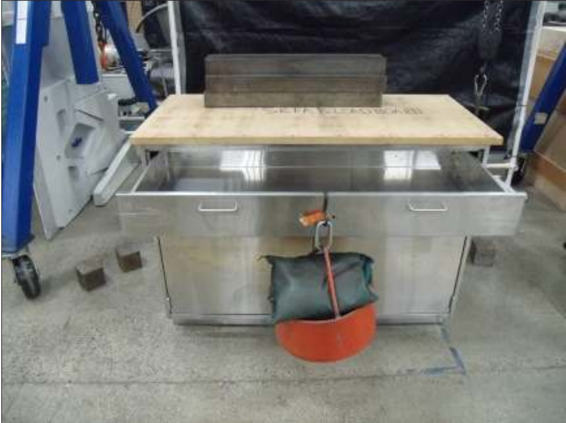
Drawer Static Load Test
