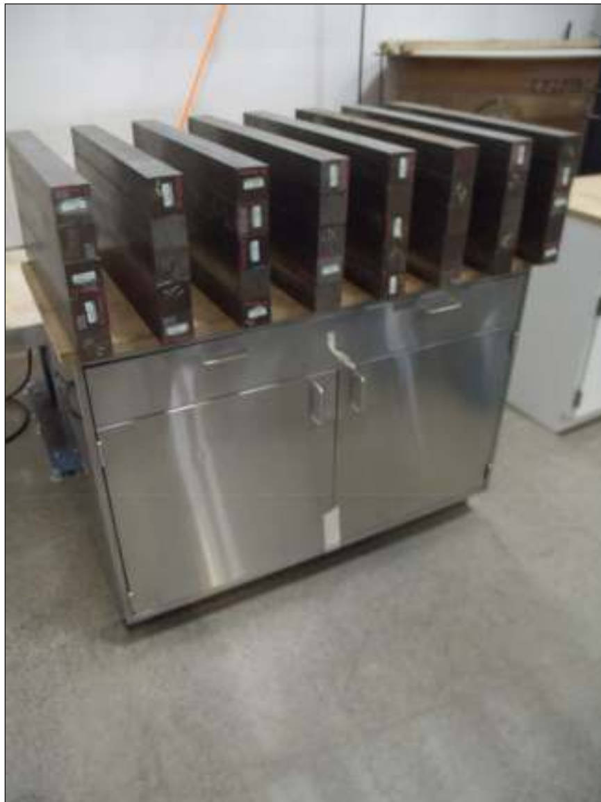
Cabinet Load Test
