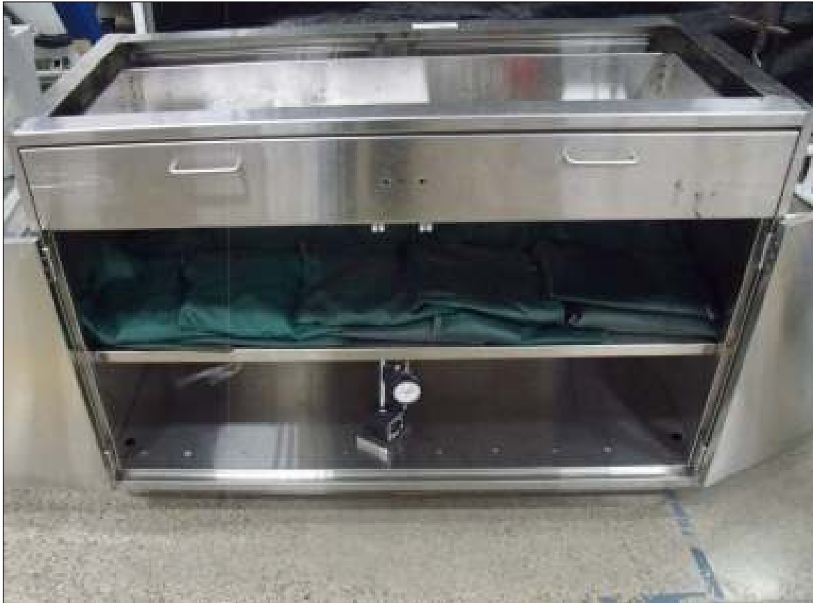
Shelf Load Test – Base Cabinet
