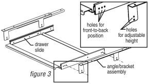
Note: Eagle worktables with channel frame come with screws (located in predrilled holes in channels) for use in mounting drawers. Otherwise, mounting hardware sold separately.
